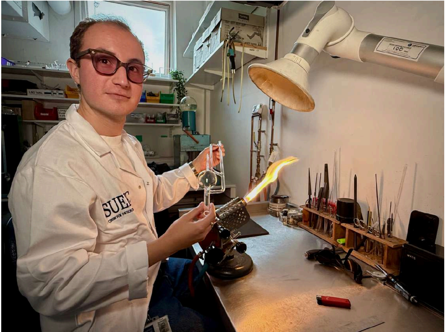
Adam Tobasnick, Technician and Glassblower at SUERC, practicing a McLeod gauge for his glassblowing exam.
