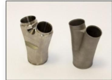
Additive layer-manufactured pipe fittings
