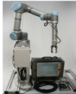
Technology for automated gauge block calibration
