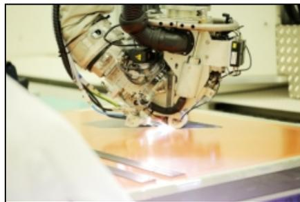
Xenon lamp pulse system for prepreg composite fibre placement
