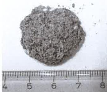
Fig. 6. Sintered mass produced in the laboratory from the reaction of marine plant ash and Stromboli beach sand.
