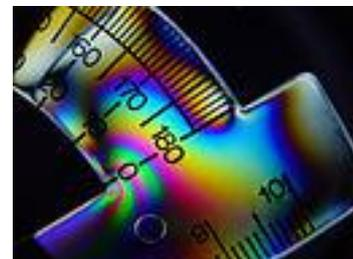
Figure 2: Protractor viewed between polarizers. [Image: CC BY-SA 3.0 via Wikimedia Commons]
